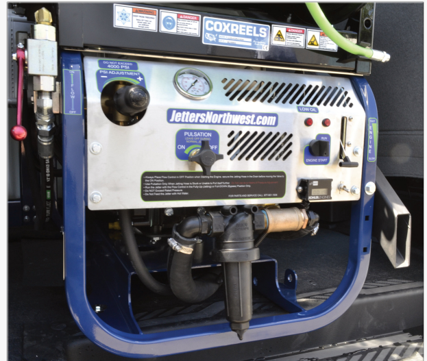
Panel Mounted Controls for easy, safe control of flow on/off and pressure adjustment
